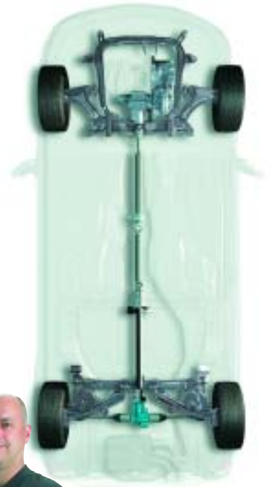
(above) AAM has the capability to design, develop and manufacture driveline components and systems for 4WD/AWD passenger cars and crossover vehicles
