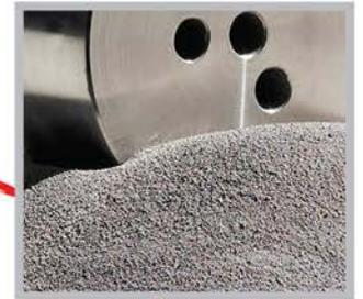
The capsule is HIPed using high temperature and pressure, fully densifying the powder metal and bonding it to the steel bar, creating a coating (cladding).
