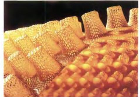
A three-dimensional braid of plastic fibers is a potential material for light-gauge construction. The highly ductile burlled pattern is an ideal base structure for the production of light-weight but very solid parts, even with complicated shapes.
