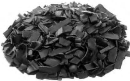
Painted polycarbonate car bumpers are ground in preparation for qualified processing. The high-grade stripping of the polycarbonate chips results in a plastic that is reprocessed into high-grade recycled materials.
