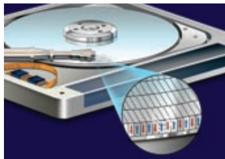
Perpendicular magnetic recording (PMR) holds more bits of data on a hard disk drive by utilizing vertical magnetic recording rather than the conventional horizontal technology. WAM materials are supporting the move to PMR.
