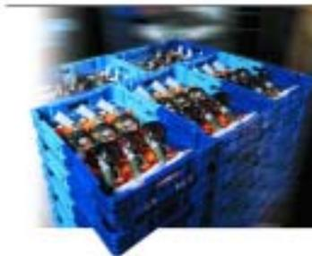
*Bi-color material handling totes allow easy sequencing of specific products on assembly lines. The reusable containers provide superior protection of delicate parts and eliminate cardboard box waste.*
