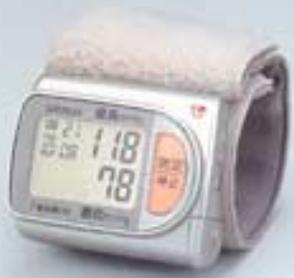
The HEM-630 is the world's smallest and lightest blood pressure monitor, and encompasses advanced sensing and fuzzy control technologies.
