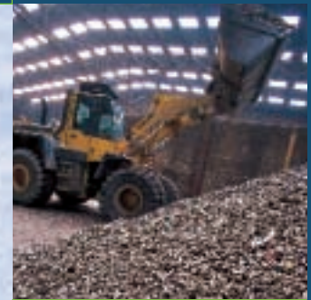
Above: Icovia's "Icopower" process produces 50,000 tonnes/year of pellets from selected waste, replacing coal as power station fuel.
